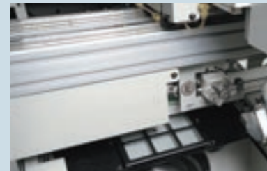
Loader capacity: \phi 50 mm x L 50 mm, 0.5 kg x 2 Max. Feed rate: X-axis 180 m/min Y-axis 130 m/min Z-axis 55 m/min
